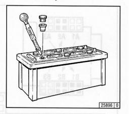
Measure the specific gravity of the individual cells with a commercial hydrometer.
